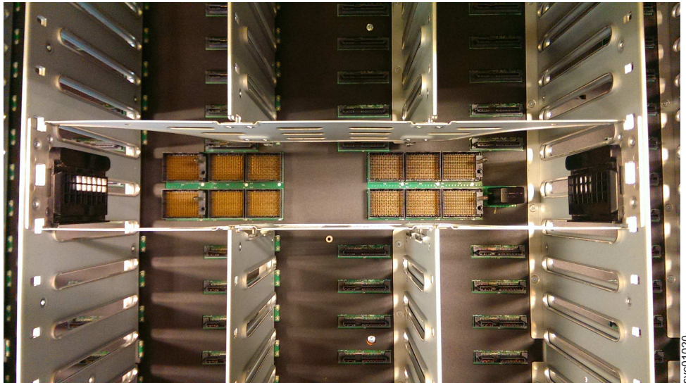
Figure 96. Secondary expander module connectors
