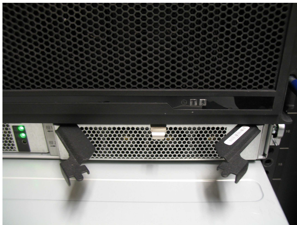
Figure 73. Install the power supply
