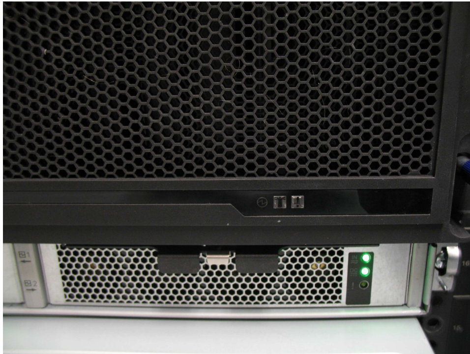
Figure 77. Fascia removed from the PSUs
