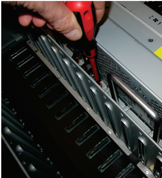
Figure 85. Secure the FIB to the drive board
