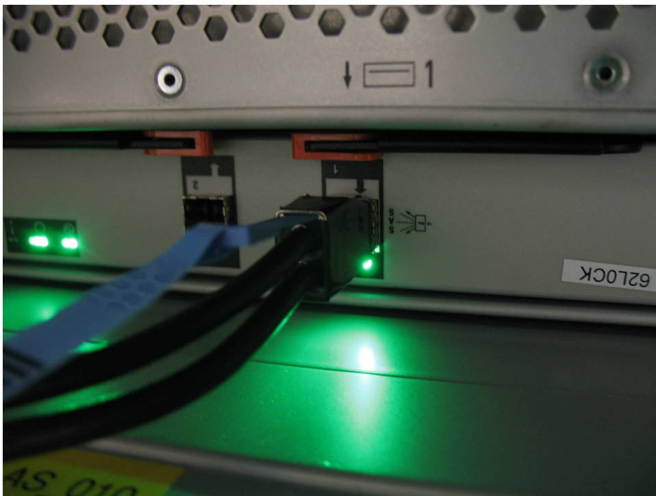
Figure 80. SAS cable correctly inserted into the SAS port
