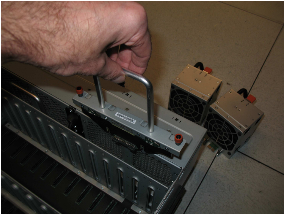
Figure 106. Remove the FIB from the chassis
