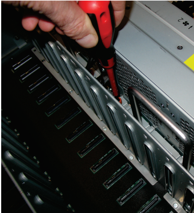
Figure 105. Loosen the FIB screws
