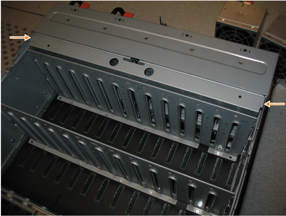
Figure 86. Replace the FIB cover
