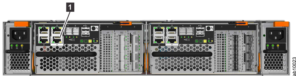
Figure 134. Storwize V7000 technician port
