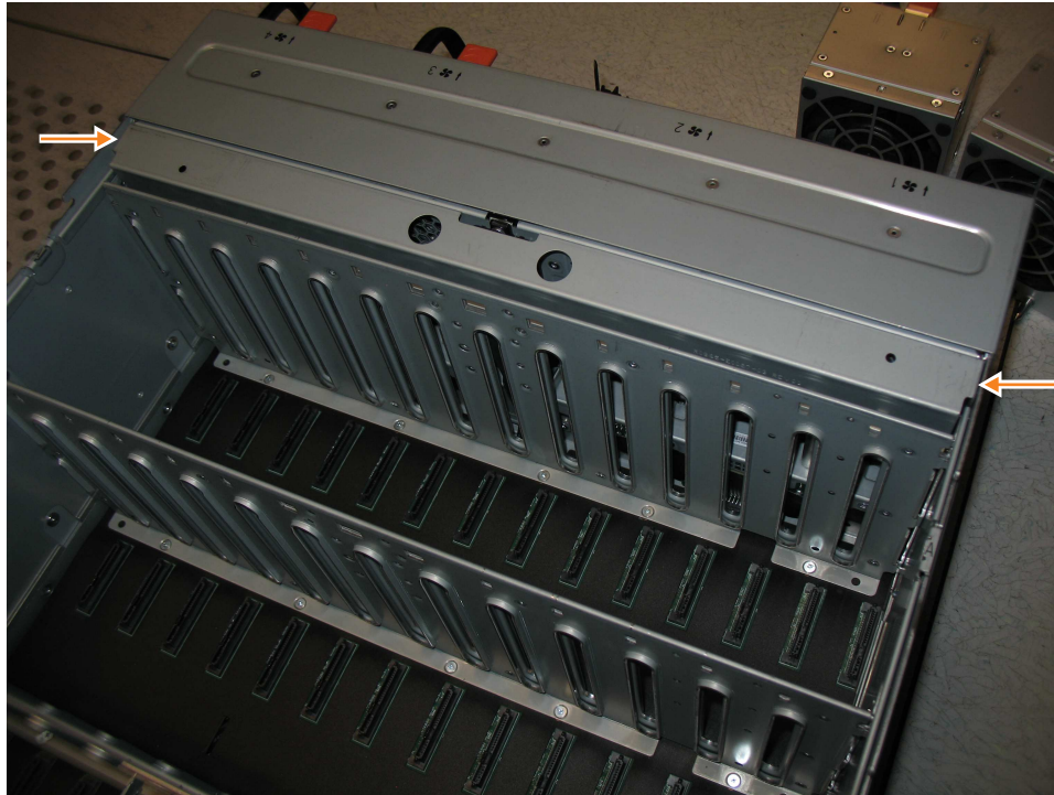
Figure 104. Location of the FIB cover
