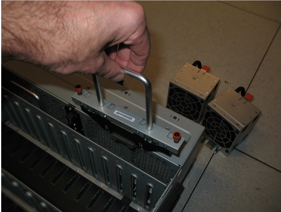
Figure 84. Insert the new FIB in the chassis
